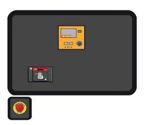
ComAp Intelilight or LOVATO ELECTRIC RGK420 SA control unit with multimeter (voltmeter, ammeter, frequencymeter, hour counter and battery voltmeter). Fuel level percentage indicator. Backlit LCD display. IP44 metal box Protection fuses Emergency button ON-OFF key selector Power terminal 4P ABB TMAX-XT magnetothermal switch
